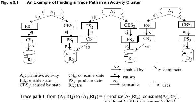
Trace path L from  $(A_3,Rt_4)$  to  $(A_1,Rt_1) = \{ produce(A_3,Rt_4), consume(A_3,Rt_3), produce(A_2,Rt_3), consume(A_2,Rt_2), produce(A_1,Rt_2), consume(A_1,Rt_1) \}$
